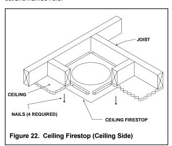
If the area above the ceiling IS an attic, position and secure the firestop on top of the previously framed hole.
